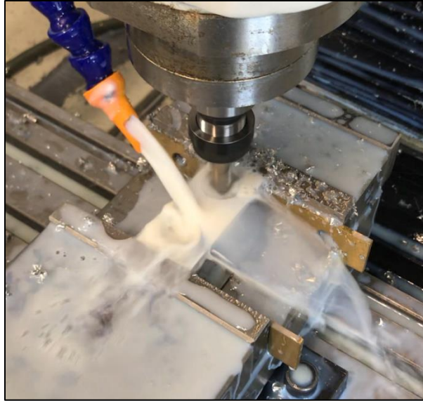
Figure 7-2: Finishing a Part on a CNC Mill
